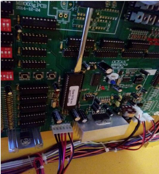
4. After you have the old programmed IC out, gently insert the new programmed IC into the slot. Make sure you line up the pins with the socket. Also notice there is a notch on the programmed IC as well as the IC socket. These notches need to line up.
