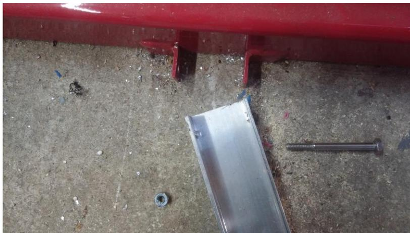
8. Attach the Sign using provided nuts, washers, and bolts.
