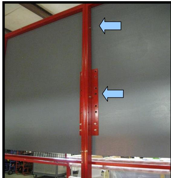
▲ Now find the top left and top right side supports and fasten them to the back panel using the 3/8"x3" Hex bolts and nuts.
