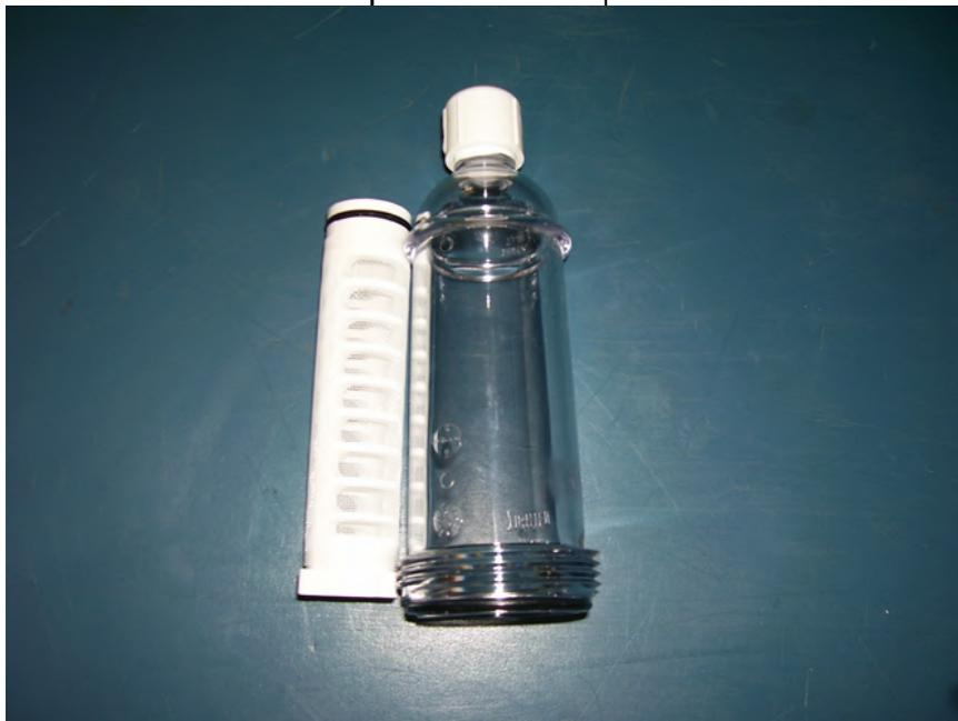
15. Carefully insert the filter cartridge into the base and screw on the bowl. DO NOT OVER TIGHTEN.
