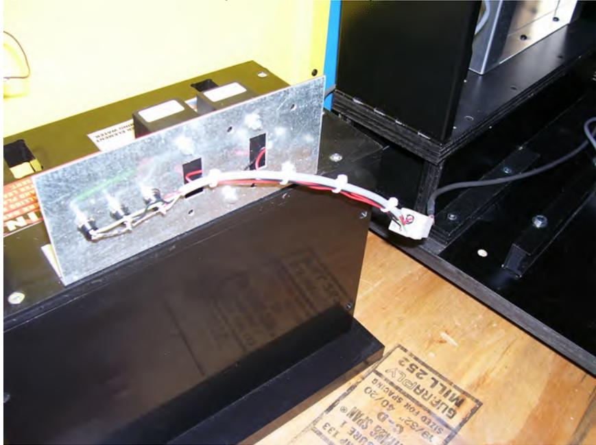
6. Slide the Pump Assembly forward. Be careful not to kink any hoses or pull any wires. (Image 4)
