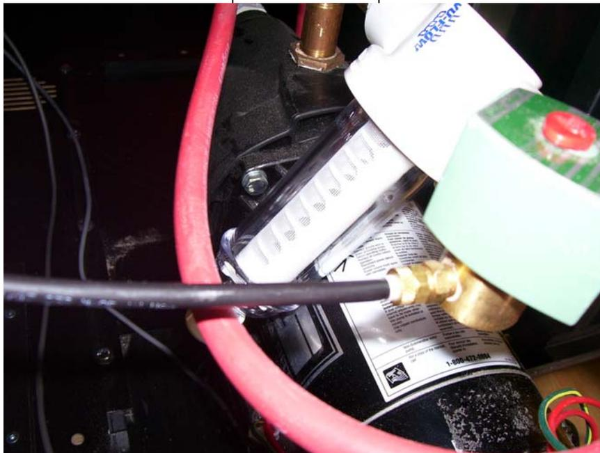
14. Clean the bowl and the filter cartridge using a soft brush and mild detergent. (Image 8)
