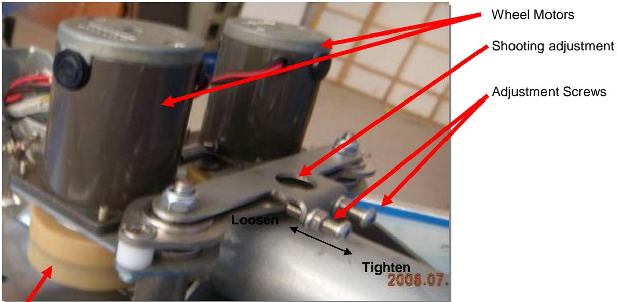
Worn wheels can cause little or no force applied to the ball. Replace if worn.
