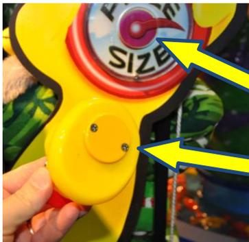
2. Operator or Customer places the RFID CHIP on the rubber duck in the provided RFID CHIP GUIDE/READER located on the duck's hand.
