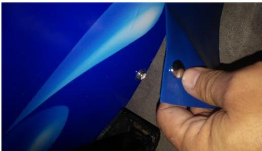
1. Install the blue skirt around the base using the provided snaps and clips.
