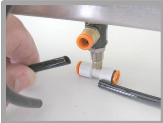
2. Disconnect air tubes from Air Valve and Tube Tee.
