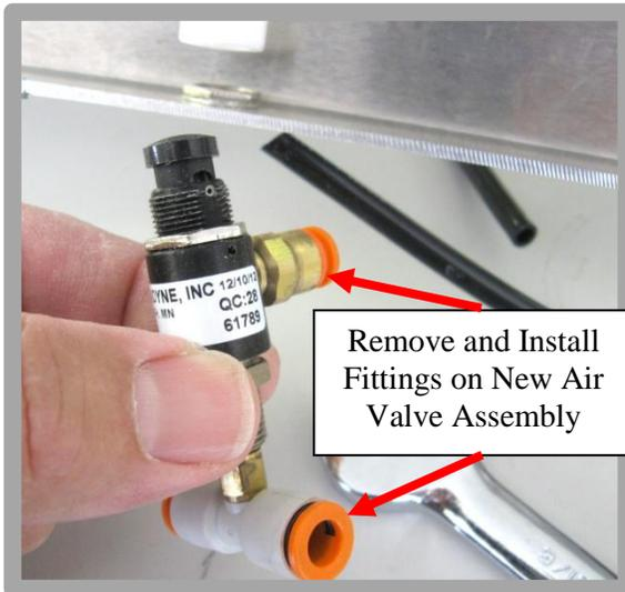
4. Once you have removed the Air Valve, remove the Tube Fitting and Tube Tee and install them on the new one.
